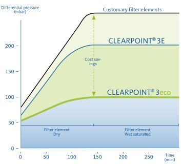
The operating costs for the CLEARPOINT<sup>®</sup> 3eco filter can be considerably lowered. The graphic illustrates them on an example of the S040 filter with filter ration S with energy-optimised volume flow.
