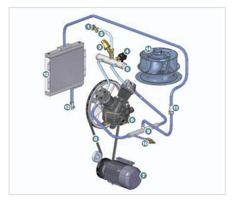
Pre-compressed air is drawn into the booster via the compressed air inlet (1).
